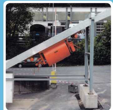
Rollover bucket in a 32° inclination = 60%
