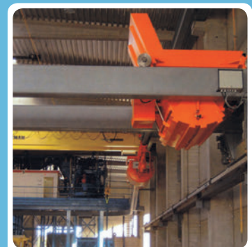
Rollover bucket and concrete distributor
